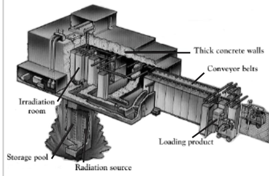
A conveyor belt carries food into an irradiation room, where it passes through a maze of stainless steel rods containing Cobalt 60.
